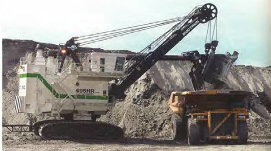
**Above:** Bucyrus model 495 electric shovel loading rock into a Cat 797B, 360-ton haul truck. The bucket has a volume of 85 cubic yards and can load 120 tons of rock in one pass, filling the truck with three scoops. (Photo: Foundation Coal Corp.)
