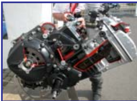
A transverse engine on a BMW!
